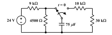
The circuit has reached the DC steady state prior to t = 0. Determine the power absorbed by the 10 k $\Omega$  resistor for  $t \ge 0$ .
